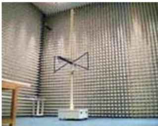
A dark room that shuts out all electromagnetic radiation
